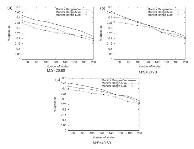
Figure 9. Comparison of speedup gain in performance between reactive and proactive bootstrapping mobility models for varying ratios of monitor and sensor nodes in the network. Mobility speed is 12 m/s.
