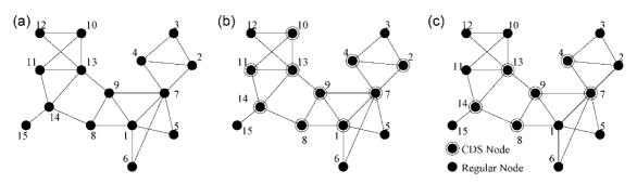
Figure 1. (a) A network of 15 nodes. (b) CDS of the network before applying *Rule-k*. (c) Reduced CDS of the network after applying *Rule-k*.
