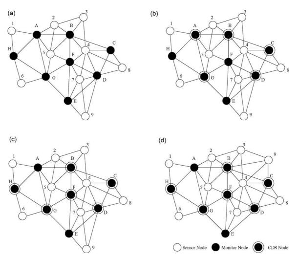
Figure 4. Hollow circles represent ordinary sensor nodes, shaded circles represent the more powerful monitor nodes, shaded circles with an outer band represent the CDS-Monitor, and the square enclosing all the nodes represents the network boundary. Mobility of nodes is confined to the square boundary. (a) Initial network, (b) CDS of the network, (c) updated CDS after monitor A sleeps, (d) updated CDS after node 9 moves to a new location and joins monitor B.
