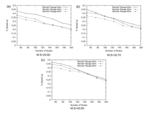
Figure 8. Comparison of speedup gain in performance between reactive and proactive bootstrapping mobility models for varying ratios of monitor and sensor nodes in the network. Mobility speed is 10 m/s.
