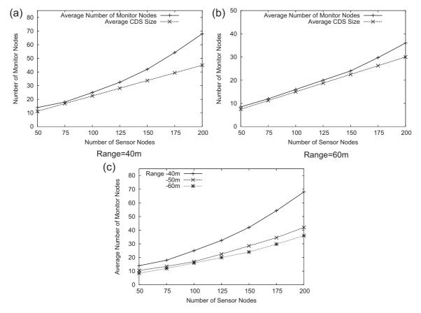
Figure 6. (a)–(b) Comparison of average number of monitor nodes with average CDS size for monitor transmission ranges 40 and 60 m, respectively. (c) Average number of monitor nodes for varying numbers of sensor nodes for varying monitor ranges.
