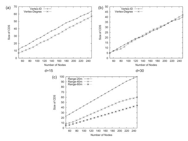
Figure 5. (a) Size of CDS with fixed d = 15. (b) Size of CDS with fixed d = 30. (c) Size of CDS with range varied from 20 to 60 m.
