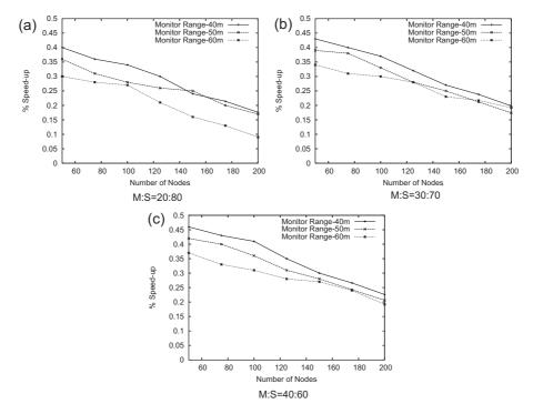
Figure 7. Comparison of speedup gain in performance between reactive and proactive bootstrapping mobility models for varying ratios of monitor and sensor nodes in the network. Mobility speed is 8 m/s.
